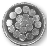
Before compression, a typical cross section of cable and lug consists of about 75% metal and 25% air.
